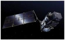
Sentinel-5 Precursor is an <u>earth atmosphere observation</u> satellite developed to close the gap in continuity of observations between Envisat and Sentinel-5
